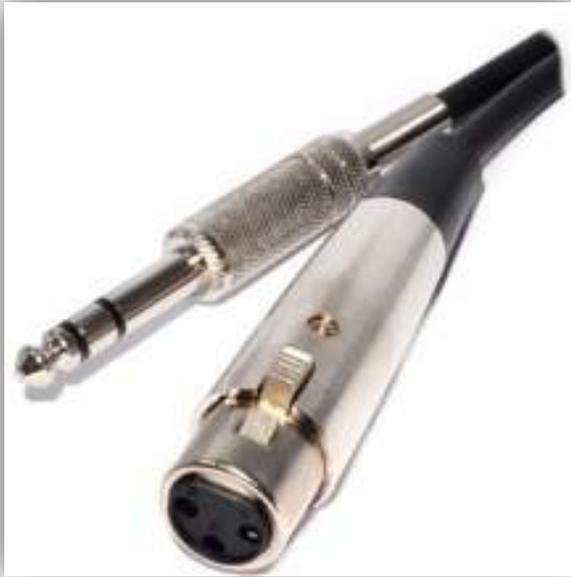
XLR connectors are usually used with microphones because of their durable construction, while TRS jack plugs are often used for mixer inputs and outputs or some monitors because of their smaller profile. (Though higher end monitors have balanced XLR inputs). TRS stands for Tip-Ring-Sleeve. These cables look like a standard guitar cable with 1/4 inch jack except they have extra rings on the actual jack
